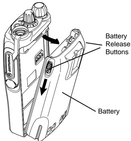
Figure 3-1: Battery Removal
