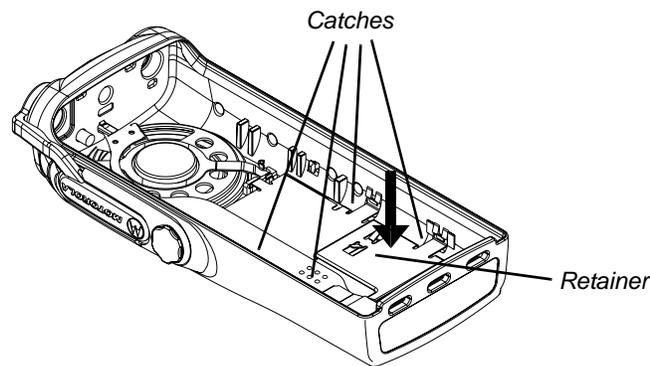
Figure 3-8: Lock Retainer Catches to the Radio's Body
