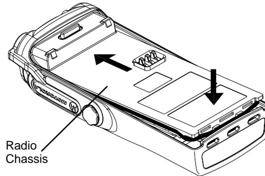
Figure 3-9: Fastening the Chassis
