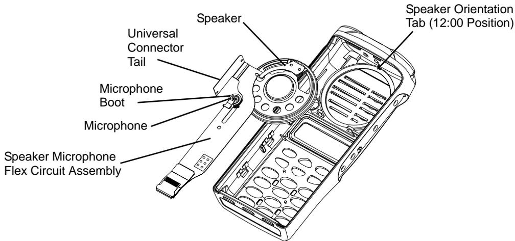
Figure 3-6: Removal Speaker-Microphone Assembly
