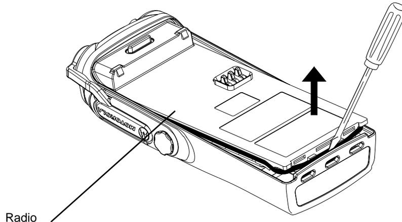
Figure 3-3: Chassis Removal
